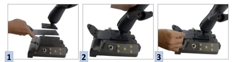
Position the sloped part of the keyboard based plate on the RAM balls (from the keyboard mounting kit), fasten four M4 x 14mm torx head screws
